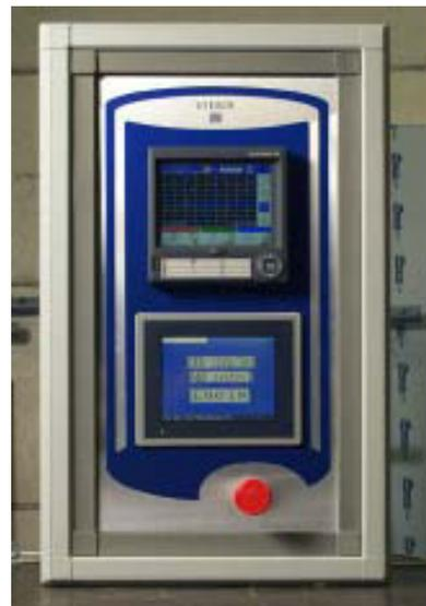
The operator interface is user friendly and easy to operate. All functions are logically grouped in menus and sub-menus to help the user navigate the screen structure with the following main menus: Decontamination, Configure, Calibration, and Service.
